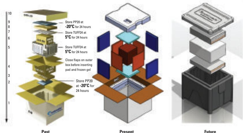
The GHPC prototype was created and adapted to incorporate 30, 25 and 15 litre payloads and cover various durations.
