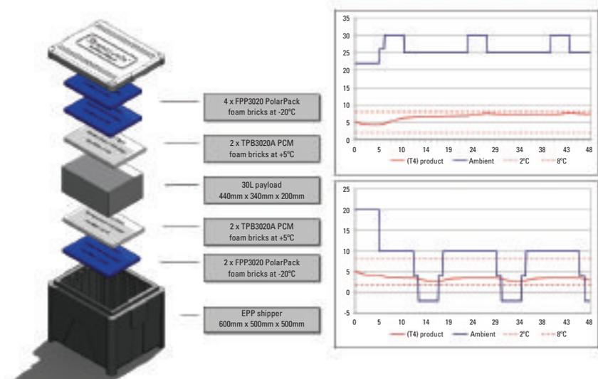
**Figure 2: Global Hybrid Platform Concept – 30L payload capacity maintaining 2-8°C for 120 hours**
